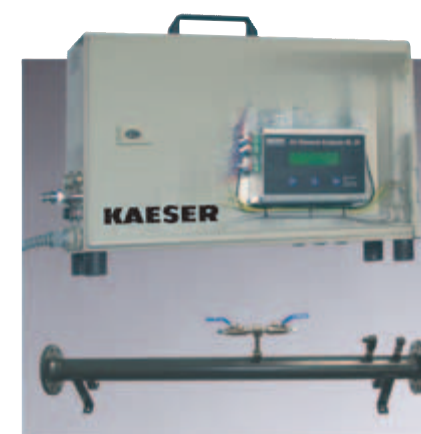
Illustration 2: Measurement of air consumption. A sampling pipe in the air main uses the pressure differential to measure flow, from which consumption can be calculated
